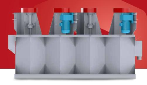
Tüfekçioğlu attrition-scrubbers, having two reverse angled propellers in each cell, produce highly efficient scrubbing and surface cleaning as a result of rubbing of grains to each other. The general use of attrition scrubbers is to open clays or to get rid of clay coatings and residues from the sand surfaces. Attrition scrubbing may rasp particles to a certain extent depending on the hardness of minerals.
